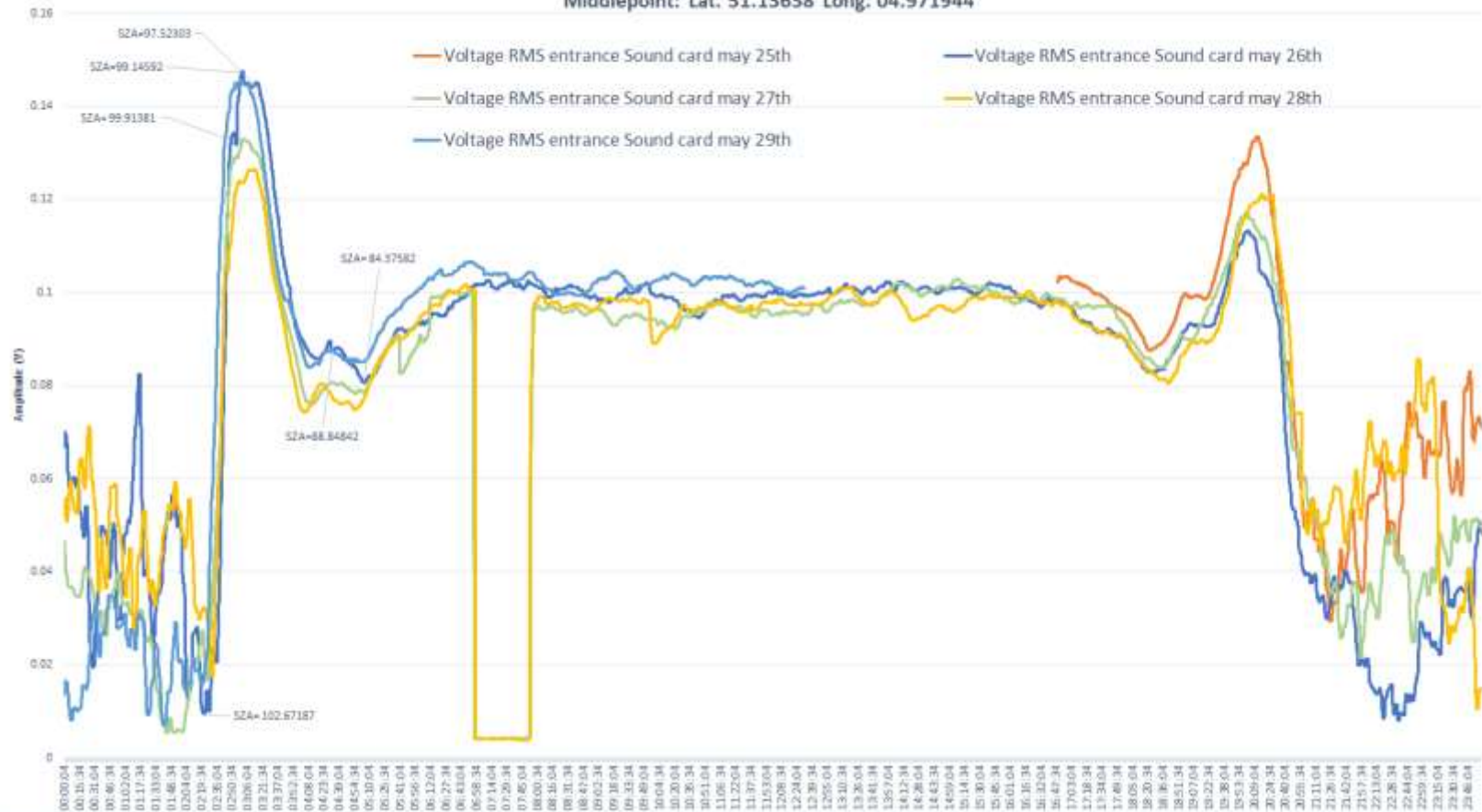
DHO38 - Volt RMS+DC Value at soundcard input - Bandwith 23,3 kHz to 23,5 kHz - Active buildin E-Field Antenna recording from May 25th to May 29th Middlepoint: Lat. 51.13638 Long. 04.971944
