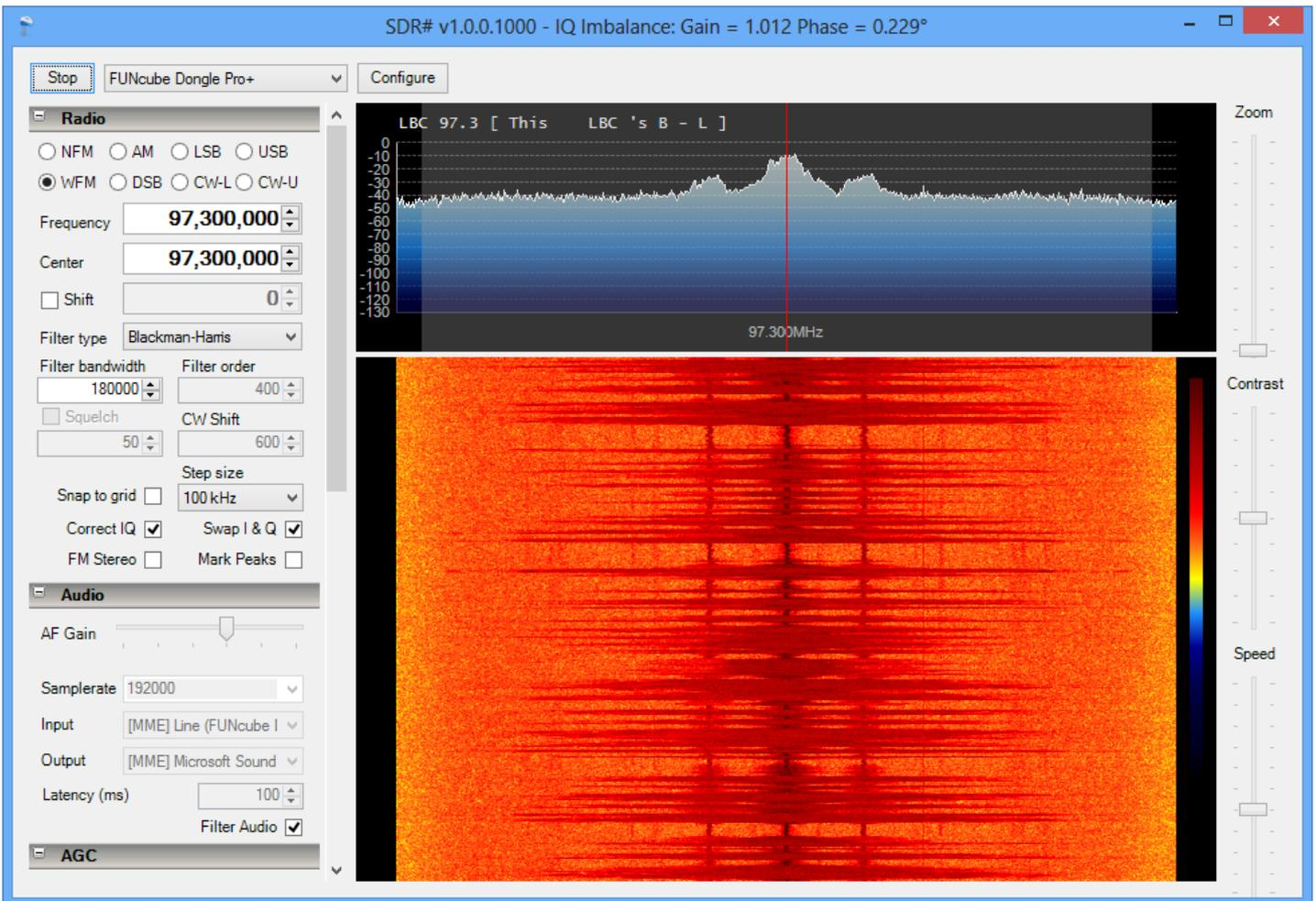
Broadcast FM is a fairly wideband signal. To receive narrowband signals such as on the AM broadcast band, set the Center frequency a few kHz away from the required frequency and then fine tune either by adjusting the Frequency setting or simply clicking on the spectrum display at the desired station. For example, below shows the reception of 909kHz on medium wave.
