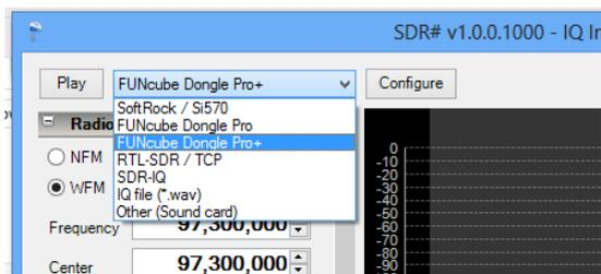
The first time you run SDRSharp, it's also wise to check some of its settings. Press the Configure button just to the right of the drop down. In particular, check that the frequency correction is set to 0.0ppm (the default is 120.0ppm).
