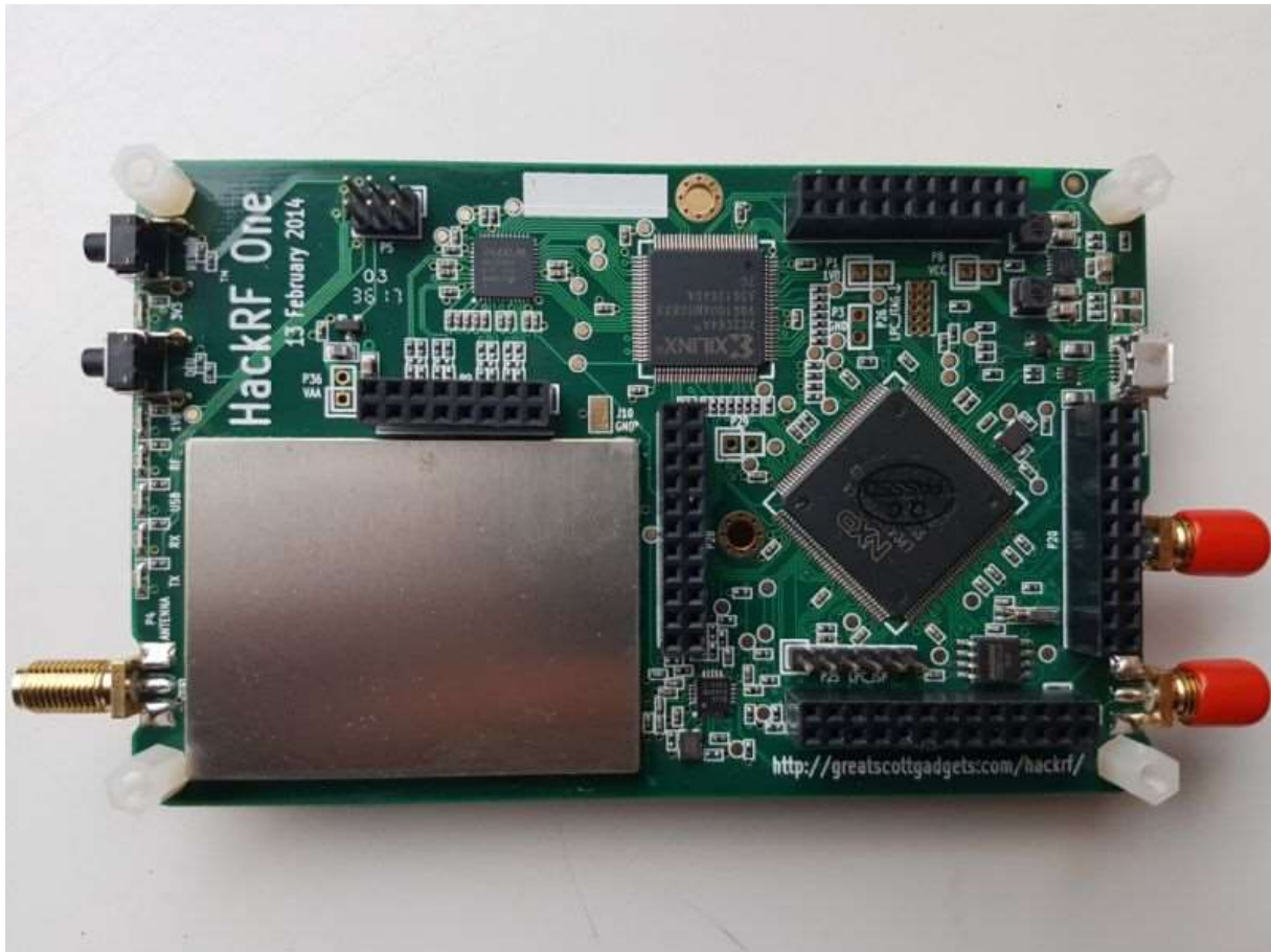
Figure 7: HackRF clone, cover removed
