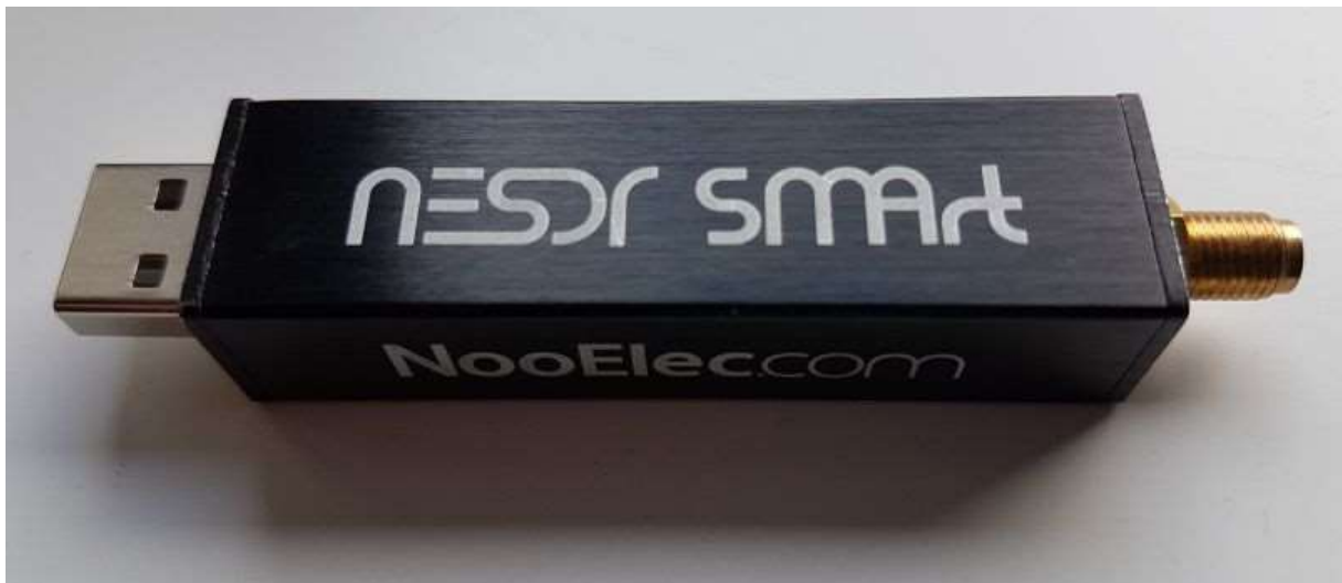
Figure 4: RTL-SDR in metal housing with SMA connector
