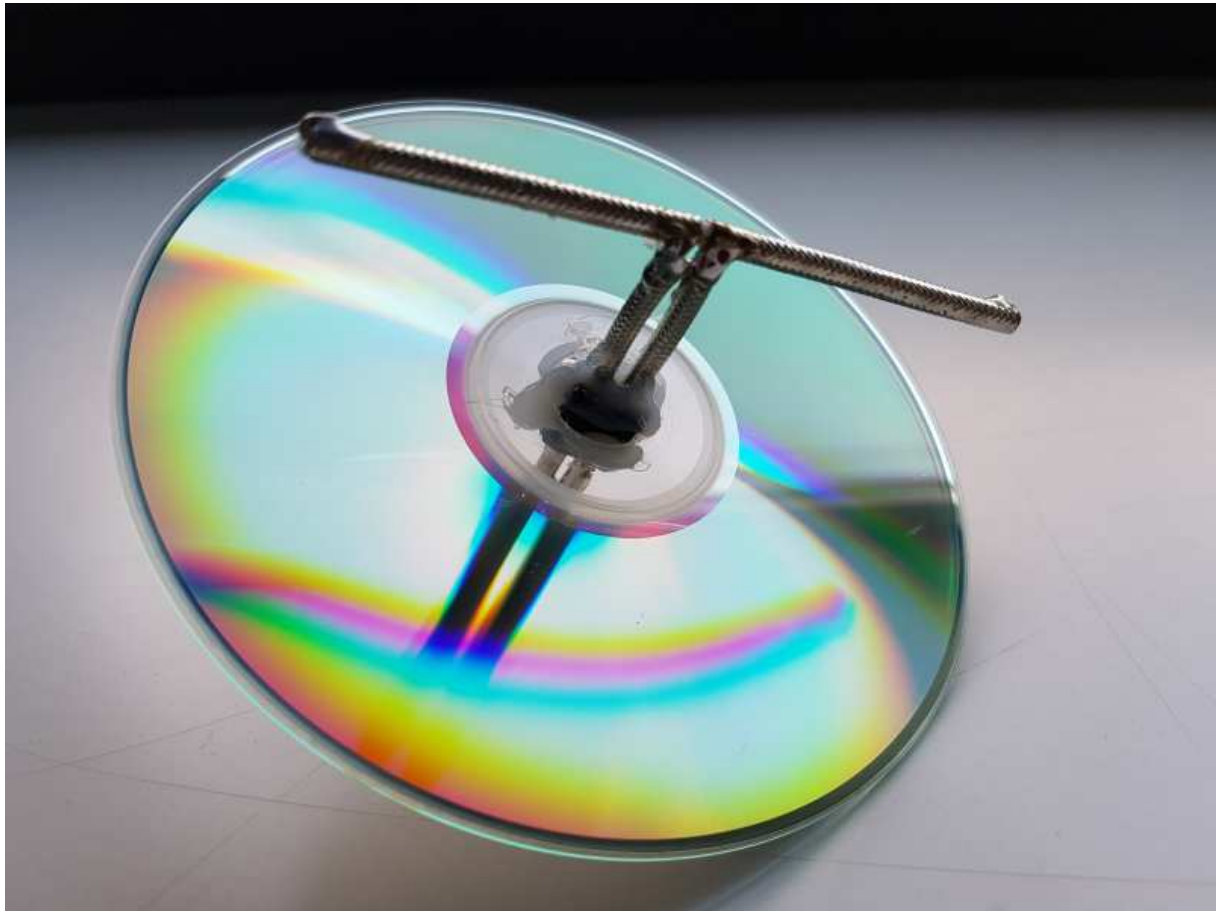
Figure 12: Dipole with CD as reflector
