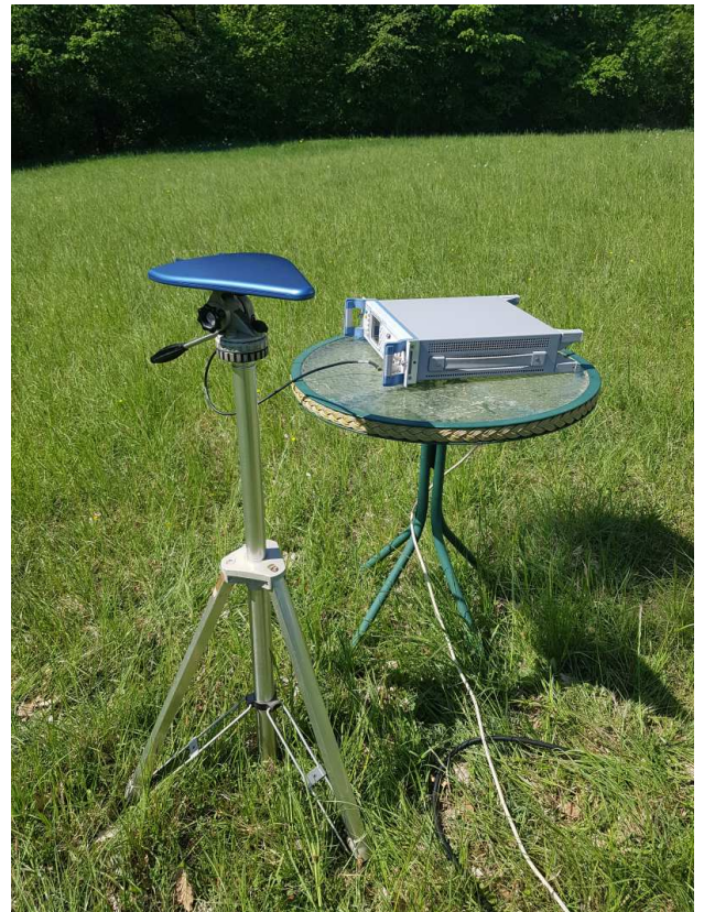
Figure 8: Photos of setup (left receive side with one of the antennas tested, right transmit side)
